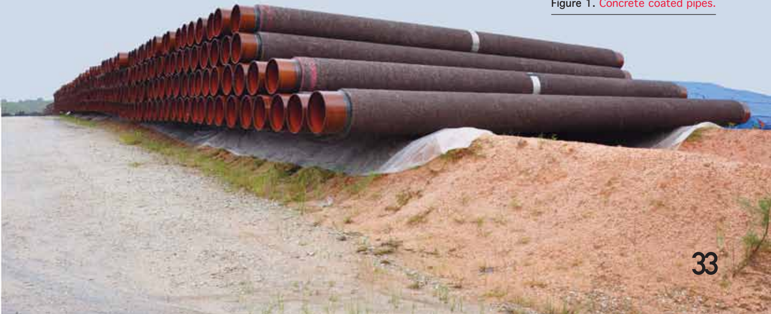
Figure 1. Concrete coated pipes.
